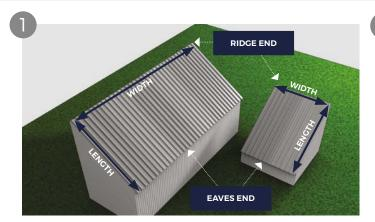
A single slope roof is sometimes referred to as a mono pitch or lean-to roof. When working out your Sheeting requirements, we require the length and width as shown in the diagram for us to be able to help you with a quotation. A width measurement is used to calculate the number of Sheets required. The length measurement is used to calculate the length of Sheets required.
