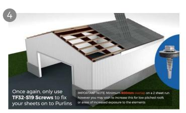
Sheets should be overlapped by the next Sheet in the run by at least one profile ('side laps'). Adjacent runs of Sheets should overlap each other by at least 600mm ('end laps'). Please note, that we can only supply a maximum of six metres. If you require a longer length, it's recommended to do a two-Sheet run.
