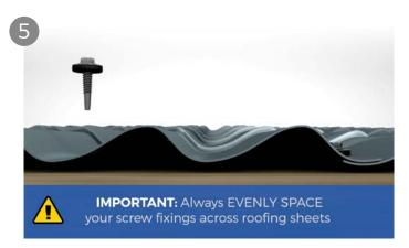
When fixing Tile Form Sheeting, it's imperative they are fixed at the valley. We recommend using TF32-S19 Screws which are self-drilling and self-sealing. Please see image above.
