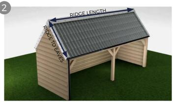
Apex roofs are separated by a central ridge. As per the diagram, we require the length of Sheet from ridge to eaves and the ridge length to calculate your requirements. You will need to measure both sides of the roof as the building/roof can vary in size from side to side. If the apex is uneven, ridge to eaves will need to be measured on both sides.
